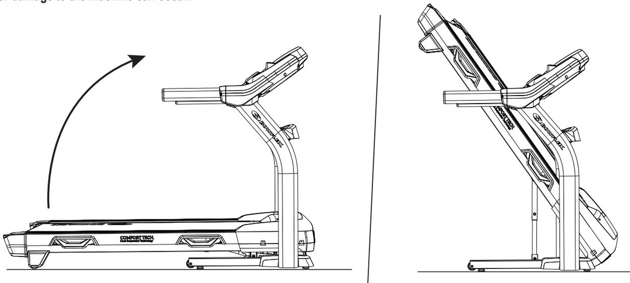
7. Make sure that the locking mechanism is engaged. Carefully pull back on the walking deck and make sure that it does not move. When you do this, keep clear of movement path in case the treadmill lock is not properly engaged.
