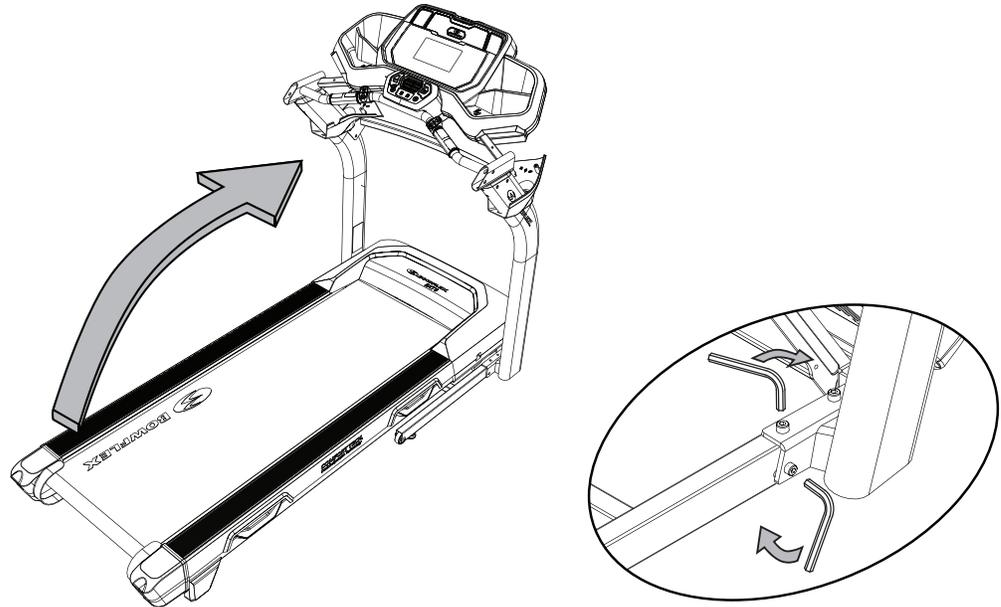
**8. Attach the Base Shrouds to the Frame Assembly, and then unfold the Walking Deck**
